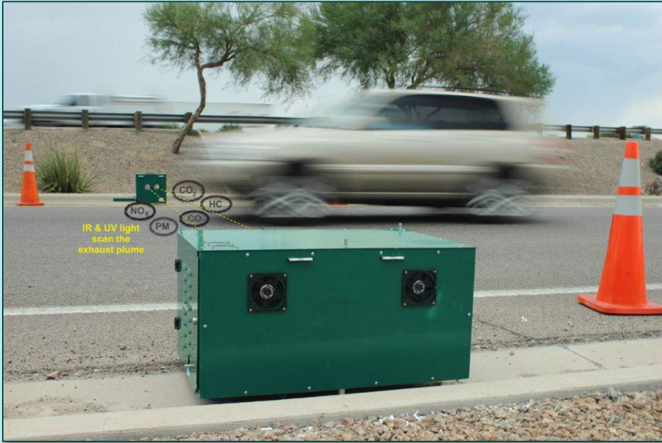
Figure 3: Unattended RSD5000s on-road deployment to measure LDVs
